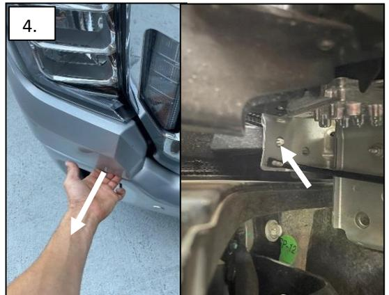
**5.** Gently pull on the grill in the areas shown to release the self locking tabs. Before removing the grill completely, un-plug the front facing camera (if-equipped).
